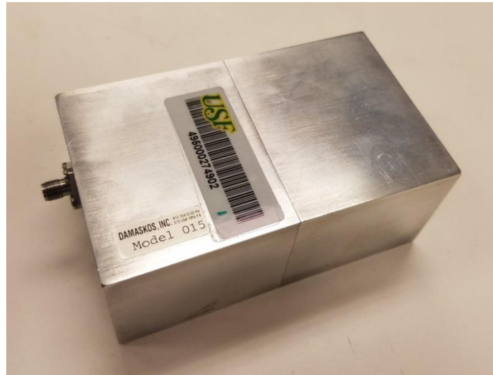
Figure A.2 - The Damaskos Model 015 Measurement Fixture used to characterize dielectric inks from 4.2-16.8 GHz at five resonance frequencies
